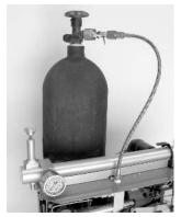
nut to fix on the tank. Check for leaks using ONLY soapy water.
