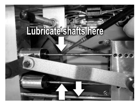
To lubricate both air pistons use **the oil you intend to extract for lubrication or equivalent vegetable oil**. Disassembly of the pistons is not required. Simply put a dab of oil on the exposed piston shafts as shown in the picture using a brush or swab. Once the unit is turned on, the oil will get pulled into the cylinder as the piston moves in and out. See our website videos on the Support page at OCOlabs.com
