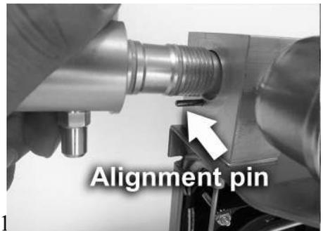
Attach the high pressure hose to the fitting on the end cap. Make sure the locking ring is seated all the way before use. Screw the knob on top of the extractor body clockwise until snug to seal up the vent.
