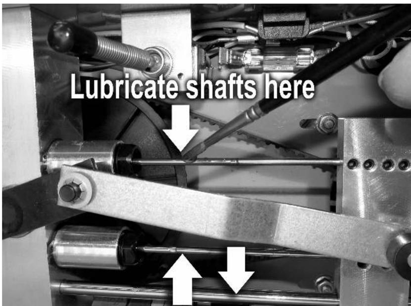
To lubricate both air pistons use **the oil you intend to extract for lubrication or equivalent vegetable oil**. Disassembly of the pistons is not required. Simply put a dab of oil on the exposed piston shafts as shown in the picture using a brush or swab. Once the unit is turned on, the oil will get pulled into the cylinder as the piston moves in and out. See our website videos on the Support page at [OCOLabs.com](http://OCOLabs.com)
