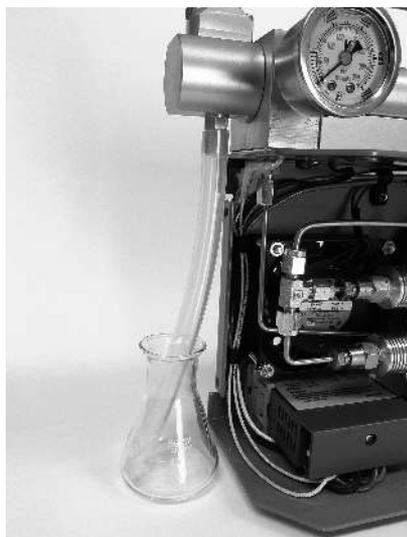
Next place the open end of the hose in the supplied flask on the table as shown. For testing, place a small amount of water covering up the end of the hose in the flask. You will see bubbles in the flask if the vent is not shut off.
