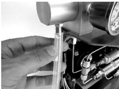
Once you have installed the extraction chamber, slide the silicone hose on the end as shown in picture.
